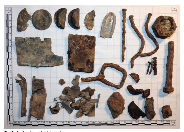
Fig. 5. Waste – iron, aluminium, zinc.
